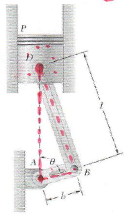
In the engine system shown,  $l = 160$  mm and  $b = 60$  mm. Knowing that the crank  $AB$  rotates with a constant angular velocity of 1000 rpm clockwise, determine the velocity of the piston  $P$  and the angular velocity of the connecting rod when (a)  $\theta = 0$ , (b)  $\theta = 90^\circ$ .
